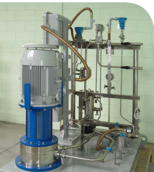
A complete RoTechBooster skid before delivery
